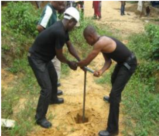
Plate 2: Hand auger boring
