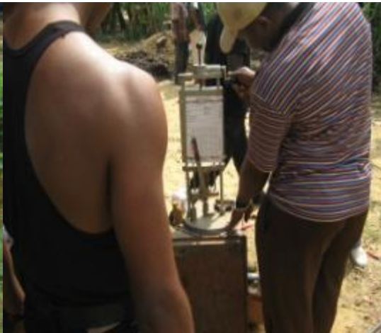
Plate 3: In-situ unconfined compression test
