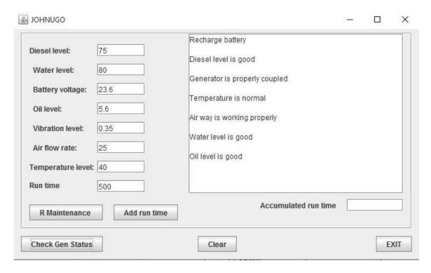
Figure 7: Operating condition of New Hostel generator
