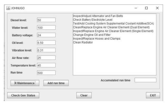
Figure 8: Recommended Routine maintenance for 500 run hours
