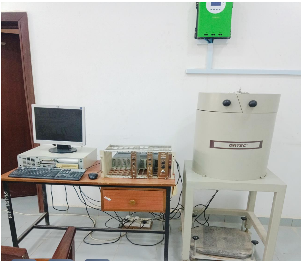
Figure 2: Picture of the CERT, A.B.U Zaria NaI(Tl) Gamma Spectrometry Section.
