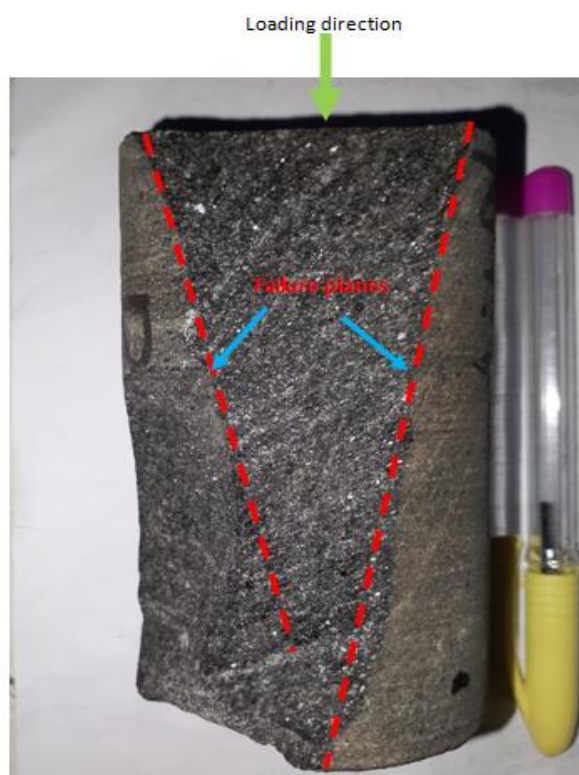
Figure 10: Vertical splitting failure in granodiorite gneiss
