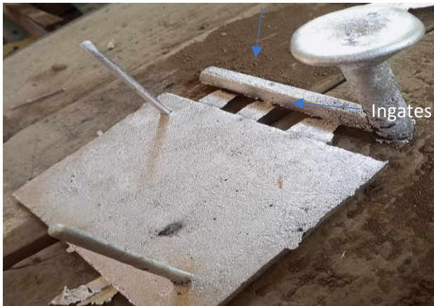
Plate 6: Product after casting with the ingate and the runner still attached
