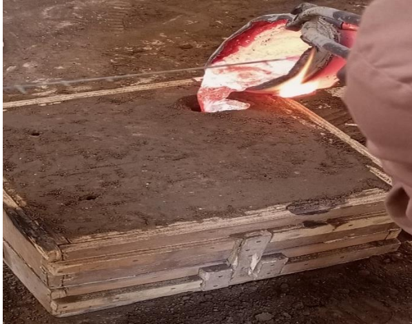
Plate 4: Pouring of molten metal into 1 st cavity
