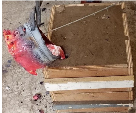
Plate 5: Pouring of molten metal into 2nd cavity
