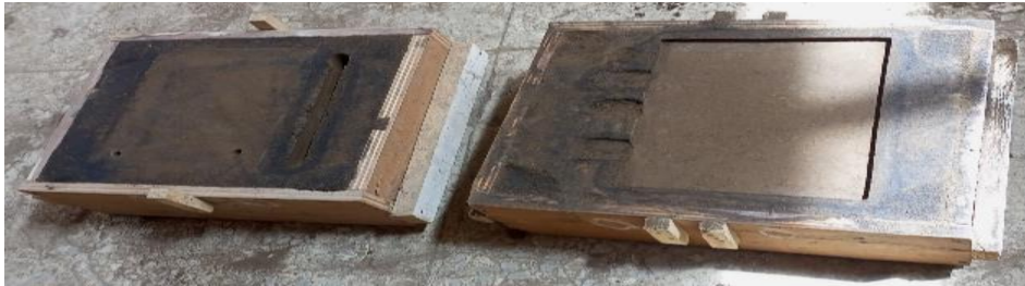
Plate 1: Sand filled cope and drag with cavity created
