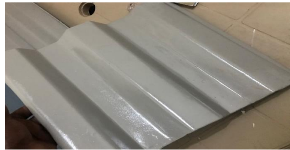
Plate 7: Completely coated corrugated sheet
